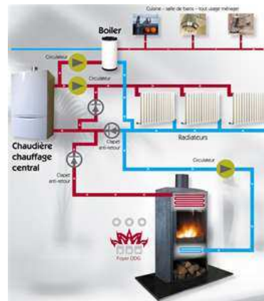
Chauffage central bois
